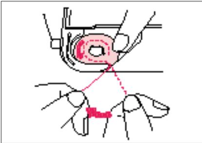
2. Insert the bobbin into the shuttle following the thread direction as noted in the etching under the bobbin cover.
