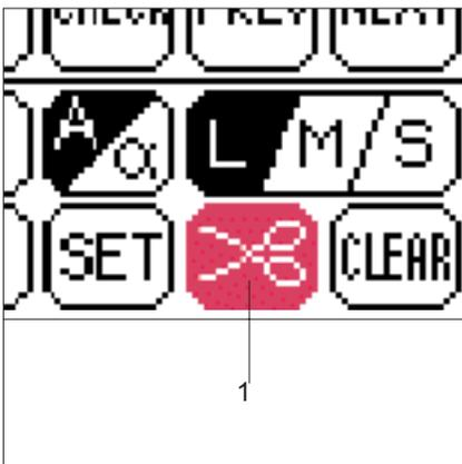
When programmed automatic thread cutting has been set, the thread is automatically cut after embroidering of each separate color is finished.
