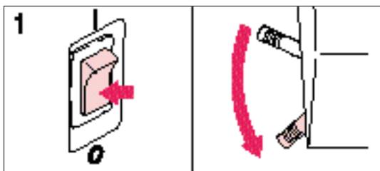
1. Turn the power switch off and lower the presser foot lever.
